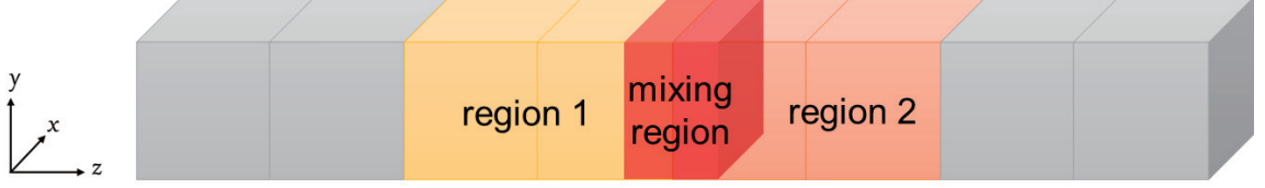
Figure 4.2: Schematic of the control volume. Quantities are volume-averaged on the mixing region (red), the left (yellow) and right (orange) sides of the mixing regions. The total volume considered is L \times L \times 4L .
