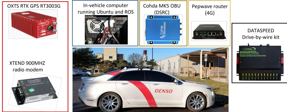
Figure 5.5: The hardware set-up of the experimental vehicle platform for POV.
