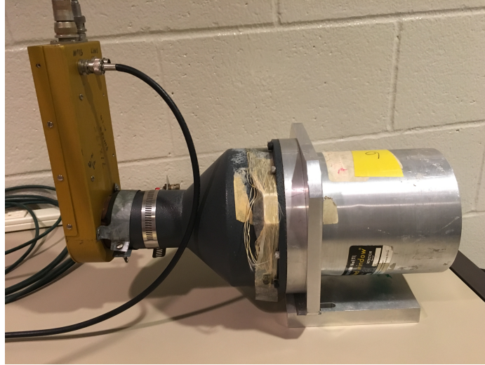
Figure 5.2: 5-inch NaI(Tl) detector, showing the preamp, PMT and NaI crystal.
