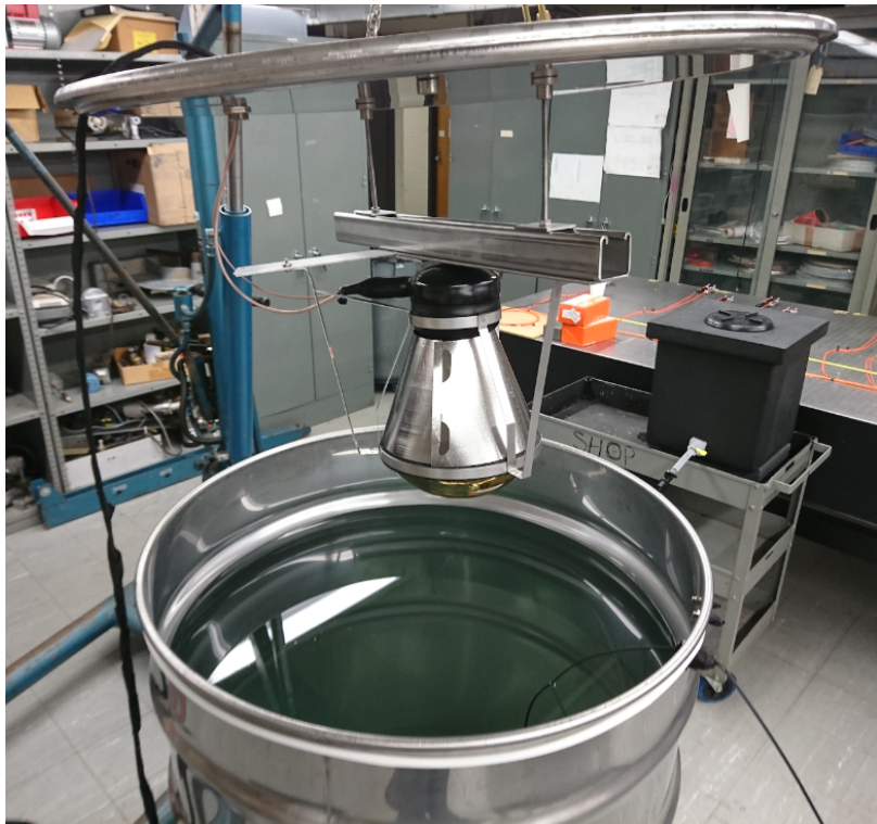
(b) OD Test Stand PMT lowered into barrel.
