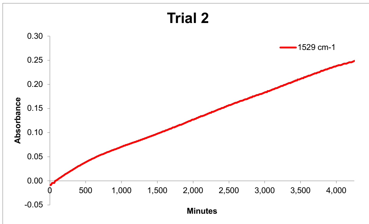
Figure C.17 FTIR kinetic measurements for the generation of product, tracked using the peak at 1529 cm -1 , for the reaction between butyl anthranilate and 2-chloroethyl isocyanate in toluene, 200 mM each.
