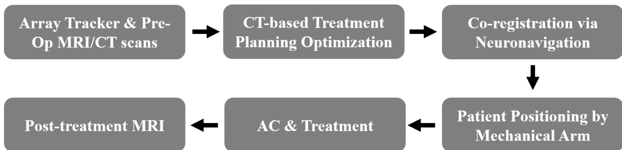
Figure 6.1. Proposed future NaviTH workflow. A new NaviTH workflow is proposed. 1) Array tracker (TTI) information and pre-operative CT and MRI images are uploaded to the neuronavigation system. From the medical images, the treatment target in the brain is selected. 2) CT-based treatment planning by ray-tracing or K-wave simulation is conducted to acquire the best
