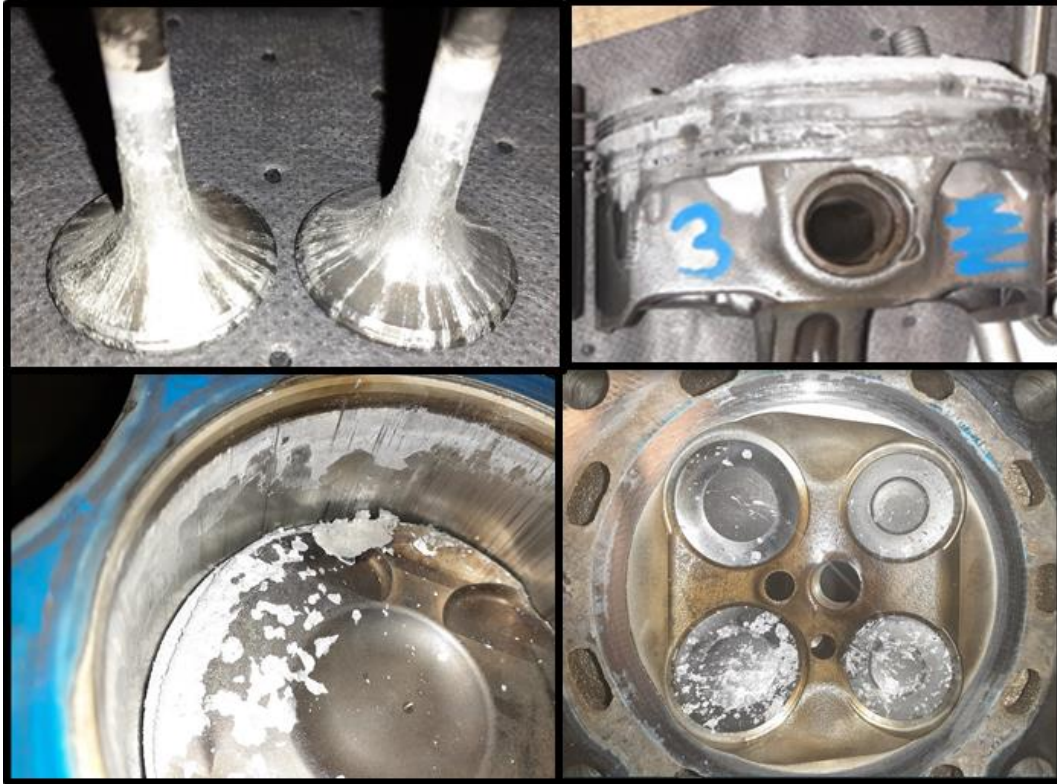
Figure 2-8: Damage to Ford Dragon 1.5L engine valves, piston, liner and head due to heavy knock event.
