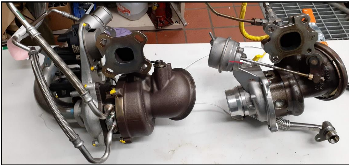
Figure 3-2: BMTS floating nozzle turbocharger (FNT) and stock Continental fixed geometry turbocharger.
