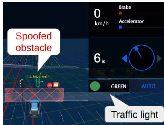
Figure 2.13: Demonstration of the AV freezing attack. The traffic light is turned green but the victim AV is not moving due to the spoofed front-near obstacles.
