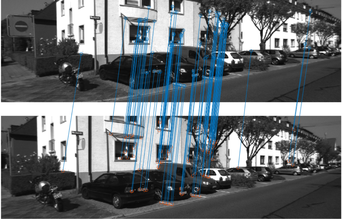
Figure 2.4: Example of the feature tracking and matching between two consecutive frames with proposed CNN feature descriptor and region-prediction based matching technique.
