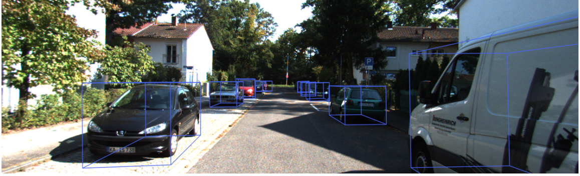
Figure 1.3: 3D surrounding object detection and localization (3D bounding box estimation) for autonomous driving cars, MVX-Net [114].
