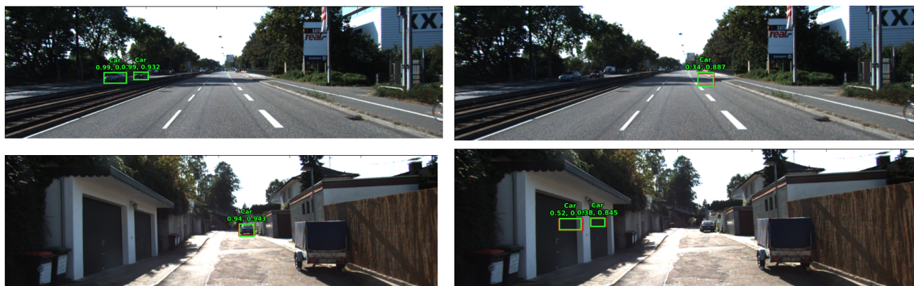
Figure 3.6: Output of experiment in which we switched LIDAR and image inputs. The two images on the left show the normal output for benign inputs. The two right images show the output when the LIDAR for one is switched for the other (and vice versa). Note that the model output follows the LIDAR (red box) more than the image.
