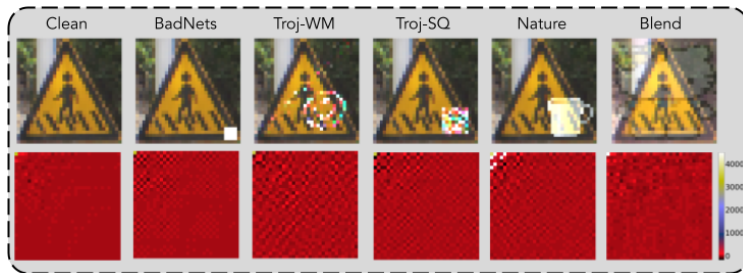
Figure 4.3: A pair-to-pair comparison of clean data and samples patching with different triggers on the TSRD database. The frequency results are averaged over all 4170 samples.
