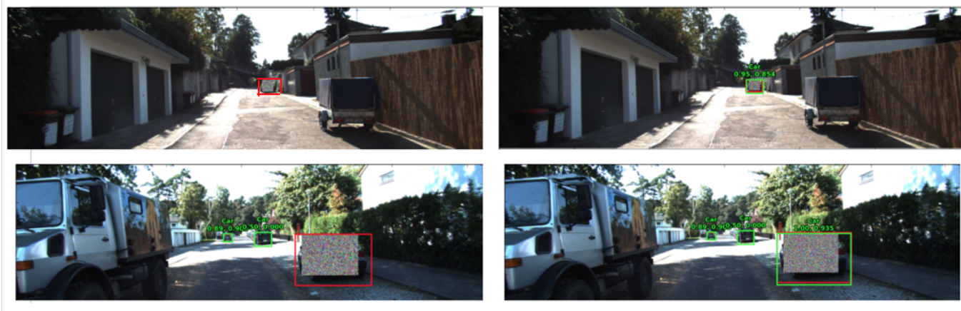
Figure 3.2: The left images are the result of the custom adversarial patch and the right images contain a random noise patch applied in the same area.
