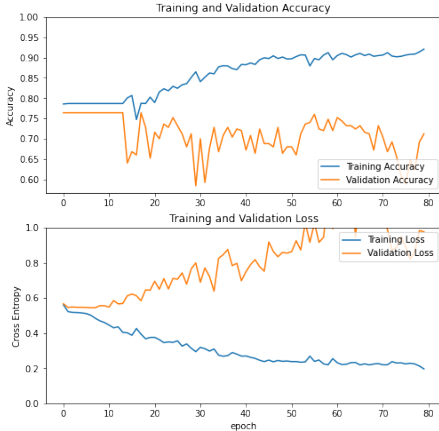
Figure 4.9: Training and validation metrics for the text-image model. Early results show parallel accuracy metrics for the training and validation data. The metrics eventually diverges, however, as the model’s parameters overfit to the training data.
