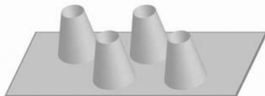
Figure 2-3 Sample Cell. The coverslip generally has 4 cut pipette tips that are glued with Epoxy to form wells that can hold a 100 \mu L sample. This design is particularly suitable for O-TIRF microscopy.
