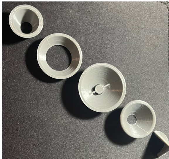
Figure 7. PLA printed prototypes of selected concepts
