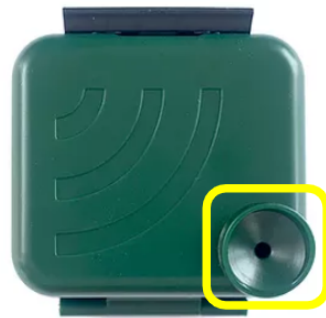
Figure 5. AudioMoth case with passive amplifier callout
