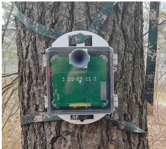
Figure 11. Final MVP with the funnel amplifier that was delivered to Backyard Brains
