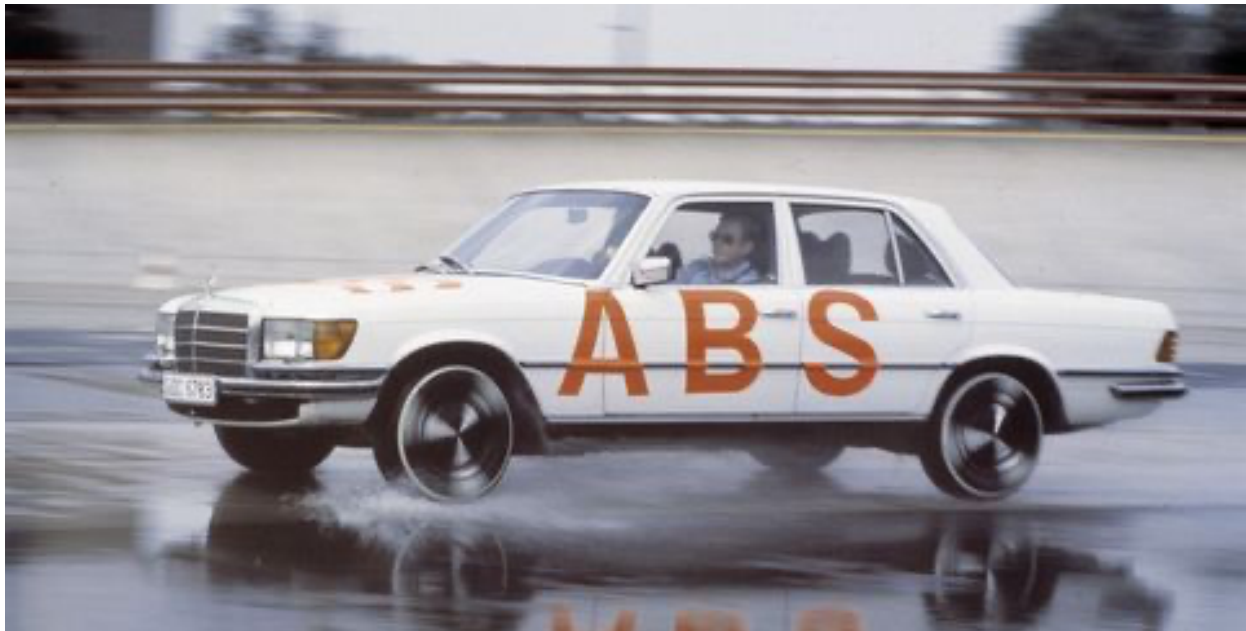
Figure 16. 1978 Mercedes-Benz W116 S-Class ABS Test Car
