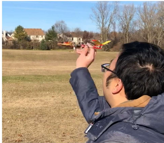
Figure 4.6. Method of launching the prototype during flight tests
