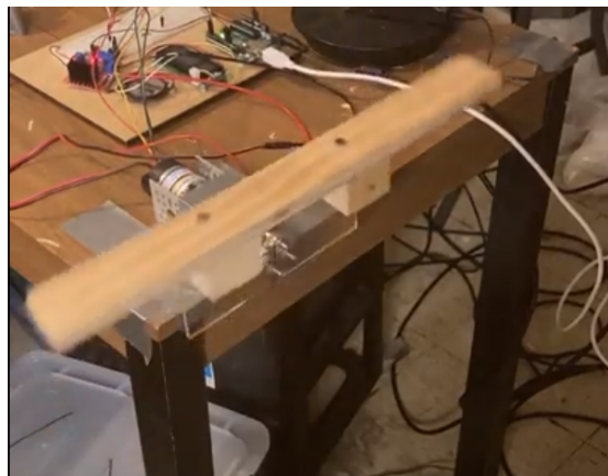
Figure 5. Hand Height measures the relative height of the musician's hands to one another
