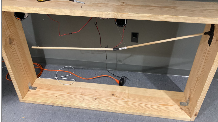
Figure 9. A smaller and more accessible Dowel Arm. The joint connecting the two dowel sticks is to be a hinge and the joint at the right is to be a ball joint.
