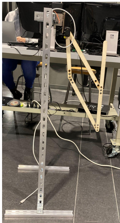
Figure 12. Final iteration of the Box on a Stick. The arm subsystem is connected to the motor mount which is at the top of the base structure.
