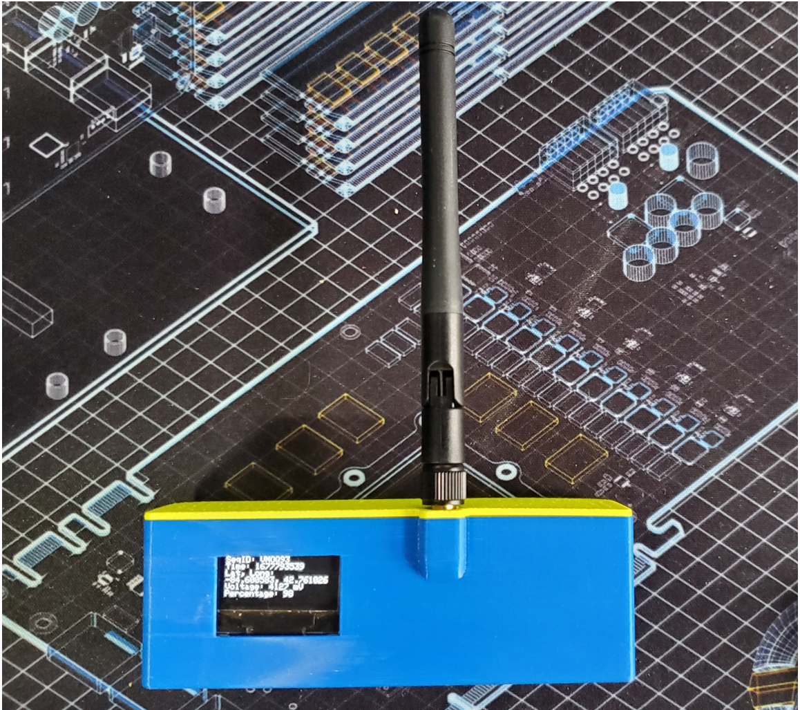
Figure 5.3: A LILLYGO TTGO LoRa module with an enclosure
