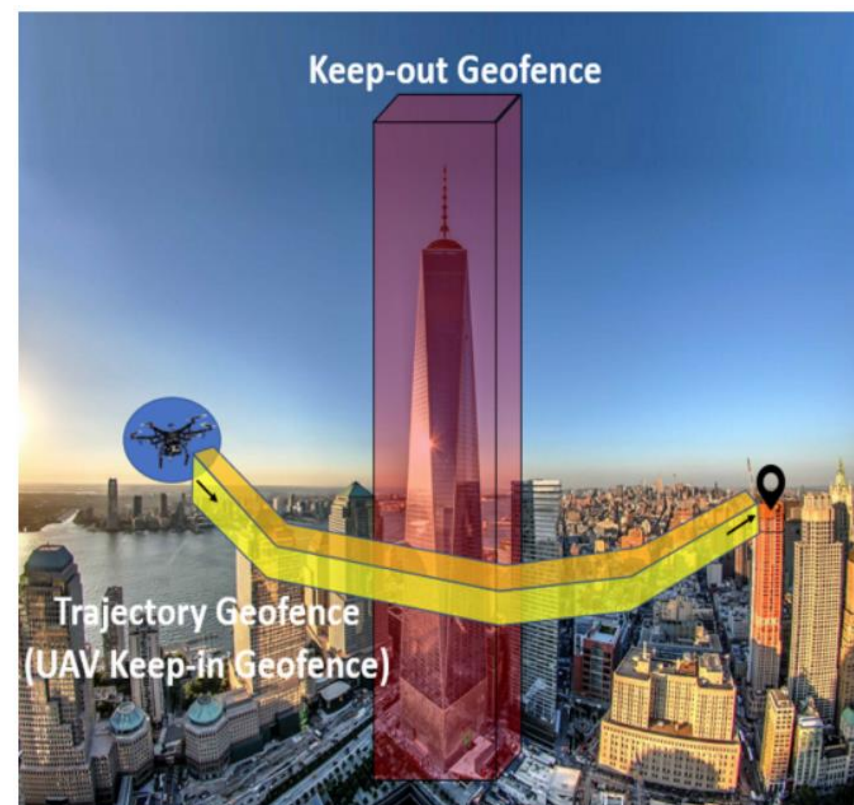
Fig. 1 Visualization of a red keep-out geofence creating a safety barrier around a building and a yellow keep in geofence creating a safety barrier around the path of a drone [1]
