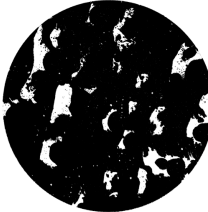
Sample 1: calculated porosity of 0.46% and no LOF observed
