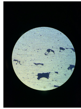
Sample 14: calculated porosity of 5.97% and LOF is observed
