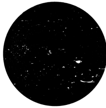
Sample 7: calculated porosity of 1.22% and LOF is observed
