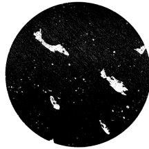
Sample 13: calculated porosity of 5.99% and LOF is observed
