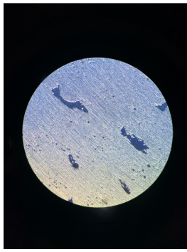
Sample 13: calculated porosity of 5.99% and LOF is observed
