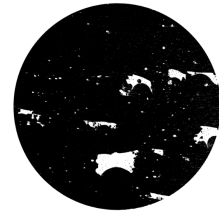
Sample 14: calculated porosity of 5.97% and LOF is observed
