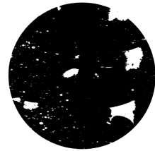
Sample 8: calculated porosity of 7.08% and LOF is observed
