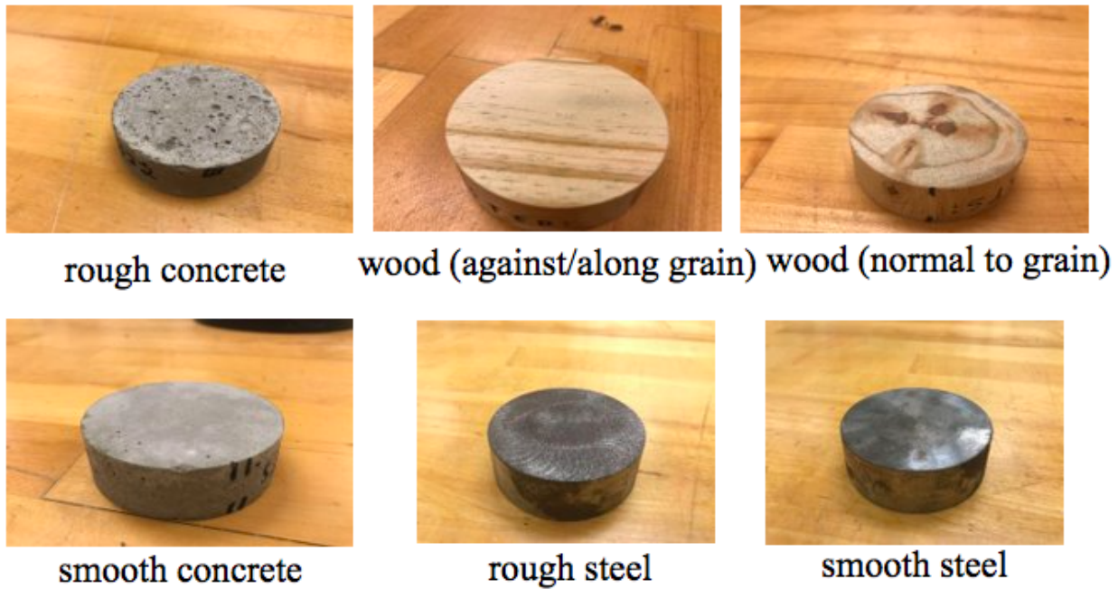
Figure 2: Different Pile Materials
