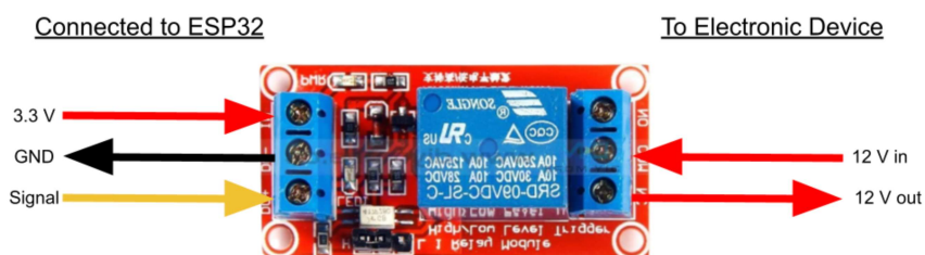
Figure 18. These relays are used throughout the prototype. The left side controls/powers the relay, the right side is powering components.
