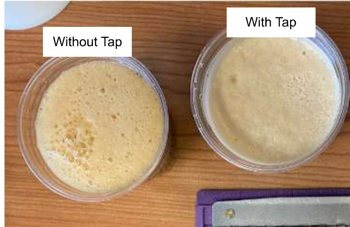
Figure 14. Tap effects on foam quality.
