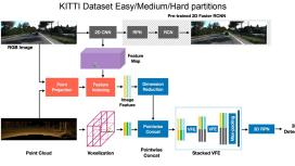
Overview of MVXNet Sensor Fusion Architecture
