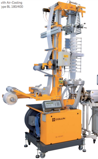
Figure 9. This figure shows what an actual pilot blown film looks like [17]. On the right of the image, pellets get fed into the extruder at a constant throughput, melted and mixed at the extruder turns, causing pressure to push melted material up through a circular die. Air gets blown into the material to create a “bubble”. At the top, the bubble flattens to create a double layered film as it’s rolled up on the core.
