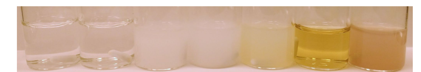
Figure 9. Demonstration of reaction sensitivity to pH indicated by color change.. From left to right: 0.5, 2, 5, 7, 9, 12, 14.
