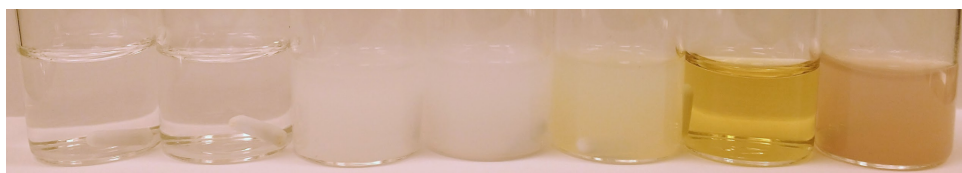
Figure 8. Demonstration of reaction sensitivity to pH indicated by color change. From left to right: pH = 0.5, 2, 5, 7, 9, 12, 14.
