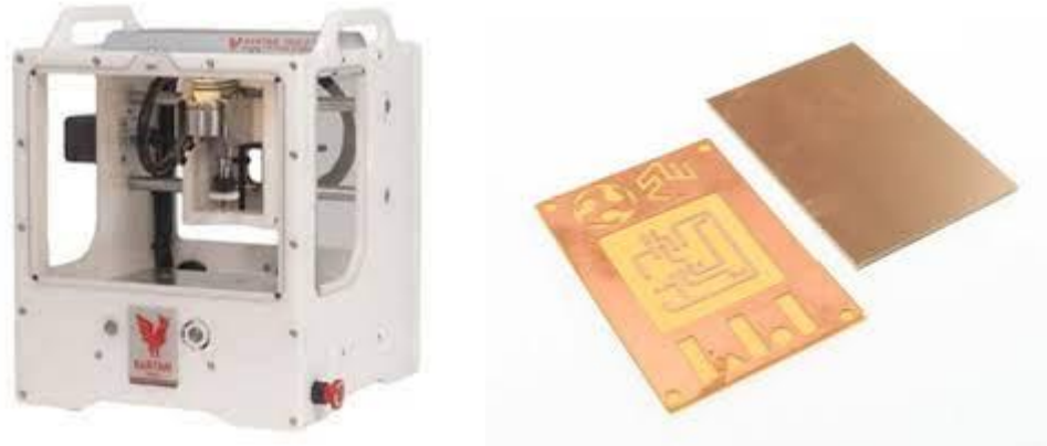
Figure 9. The Bantam PCB mill and FR-1 PCB blanks. These are resources readily available in the Duderstadt fabrication studio.
