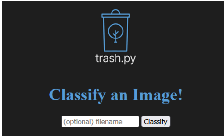
Figure 10. Landing page for trash.py web applet. If no filename is given, the image is saved in the database as item_default.jpg which is overwritten. Giving a unique filename allows the image to persist in the database.
