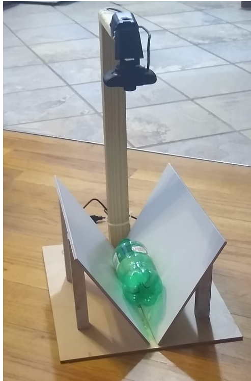
Figure 9. Prototype of the trash.py staging area. Items are held in the v-shaped area to be photographed by the camera, which points down from the top. The camera connects to a computer running the flask web server to simulate the bin's functions
