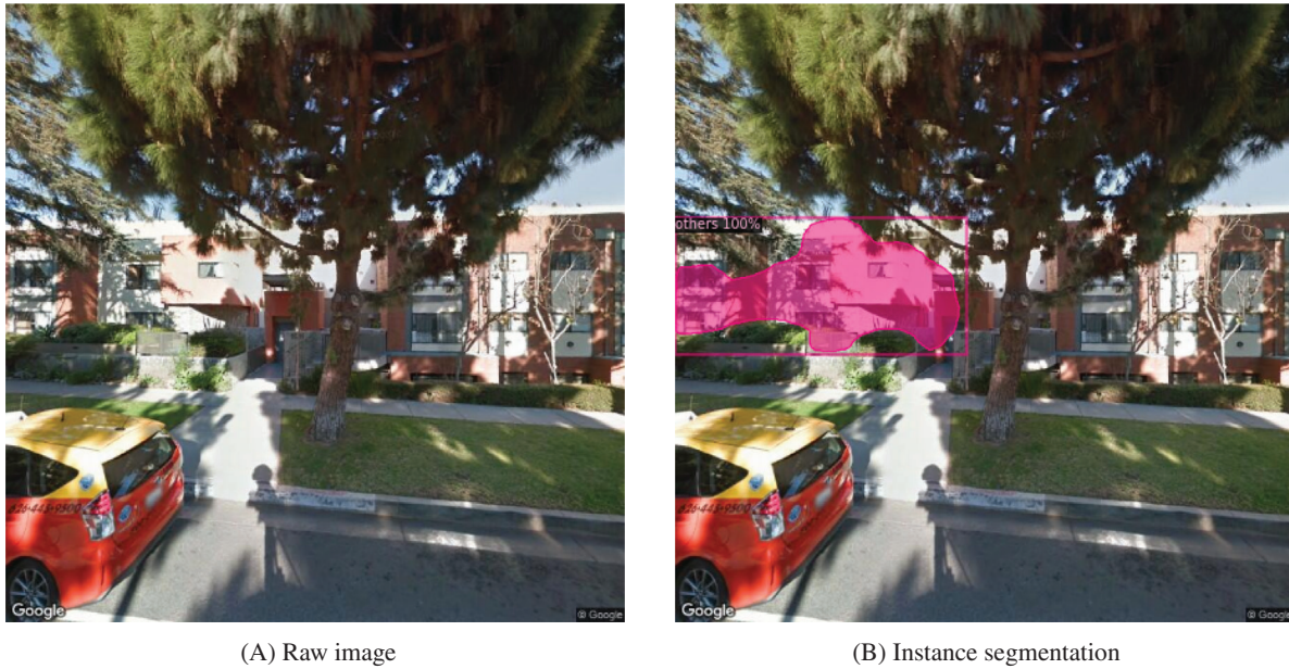
FIGURE 12 Vegetation casts complex shadows onto the building. Even though this changes the building's appearance heavily, the approach succeeds in labeling sufficient pixel and the overall building class correctly, seen in B).
