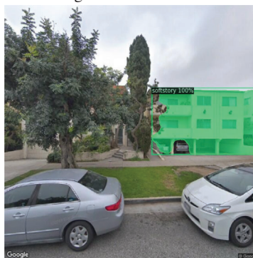
(E) Instance segmentation: there is a SS building in the image, and the location of the building is identified
