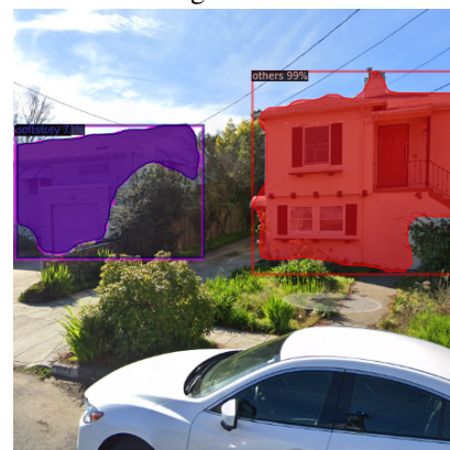
(f) Instance segmentation: there are a SS and a non-SS building in the image, and the locations of the buildings are identified
