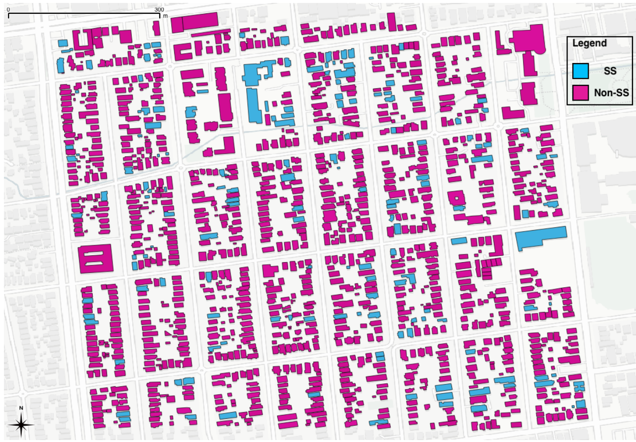
FIGURE 13 SS building detection in the Central Berkeley neighborhood, California
