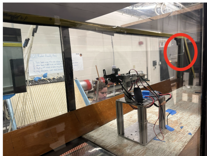
Figure 5.3: Dynamic Thrust Test Setup
