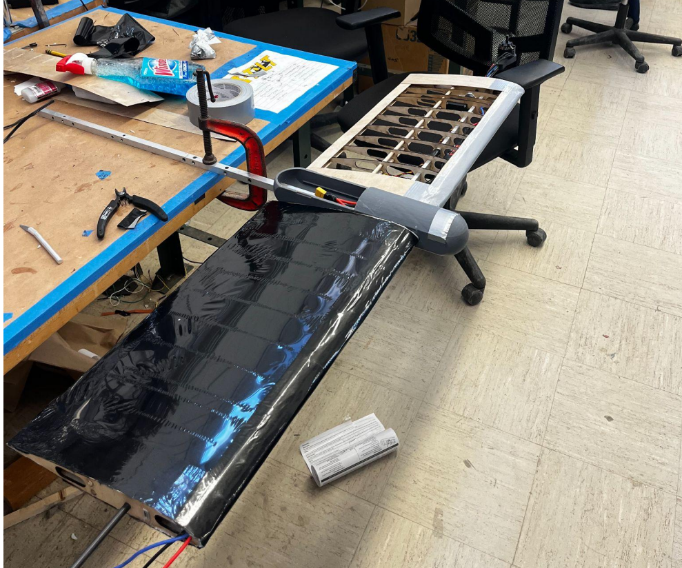
Figure A.4: Prototype Drone During Wing Monokoting
