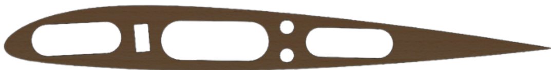
Figure A.2: NACA 24012 Airfoil with Spaces for Support Structure and Electronics
