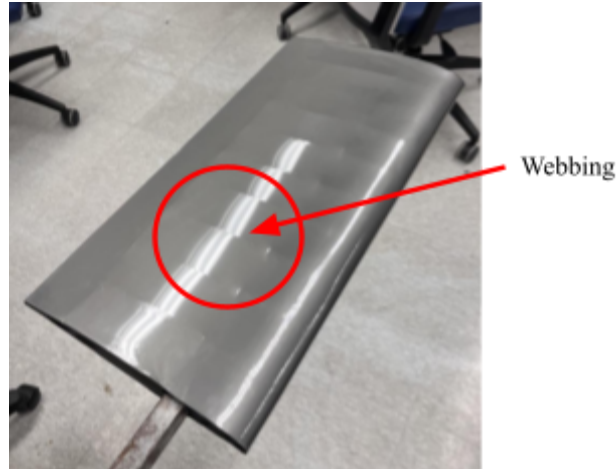
Figure B.2: Webbing Effect on MonoKote Wing
