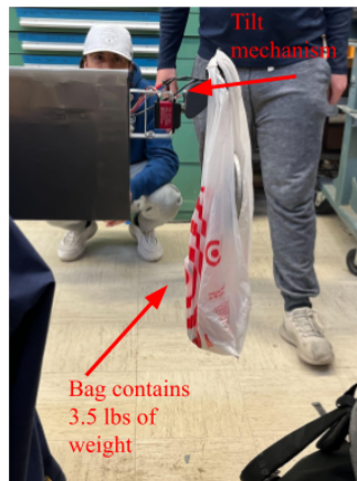
Figure 5.9: Tilt Mechanism Load Test Setup
