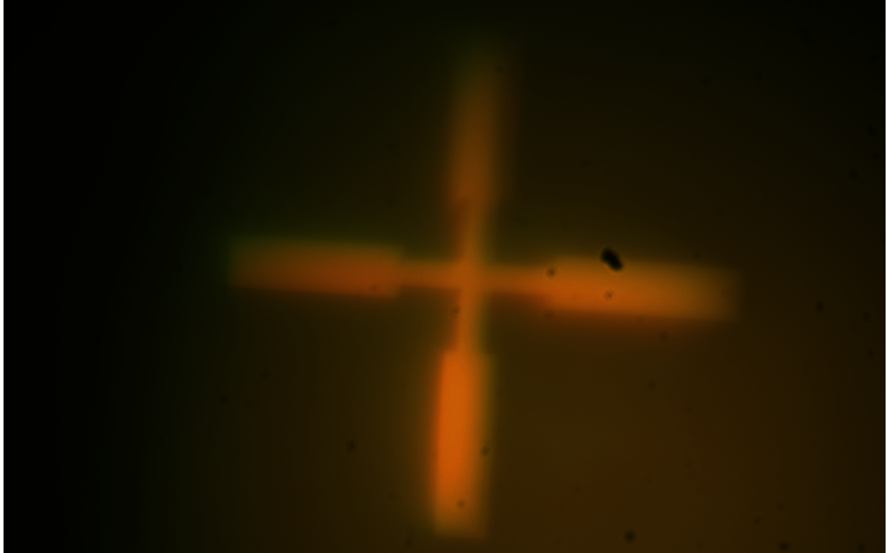
Figure 7: Patterned sample as captured by the CCD camera in the experimental setup shown in Figure 4. This pattern is approximately 100 microns across its longest dimension. Capturing a clear, crisp image of this pattern indicates that the experimental setup is sound and well-optimized.
