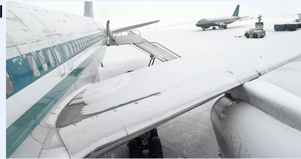
Figure 1. Hazardous ice formation on aircraft wing
