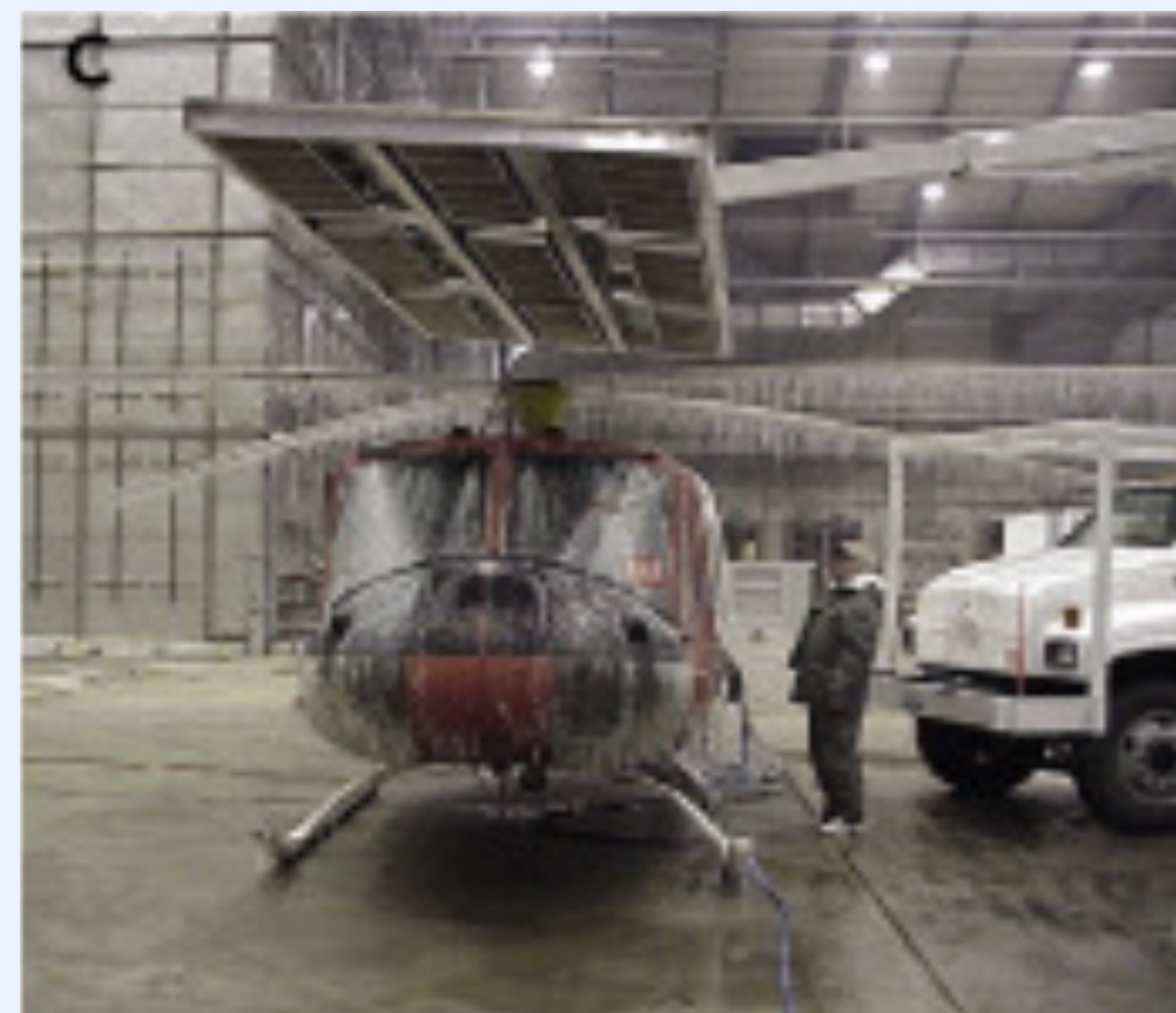
Figure 2. Electrically powered heater de-icing a helicopter from glaze ice
