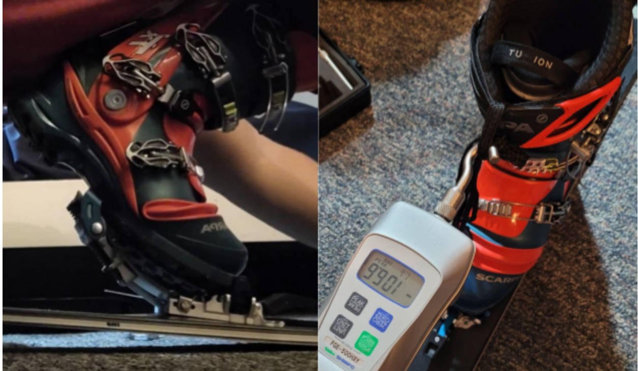
Figure 6: Shown is the apparatus used to find the force needed to flex the binding into the lunge position. Full lunge position has a nearly parallel to the ground shin.
