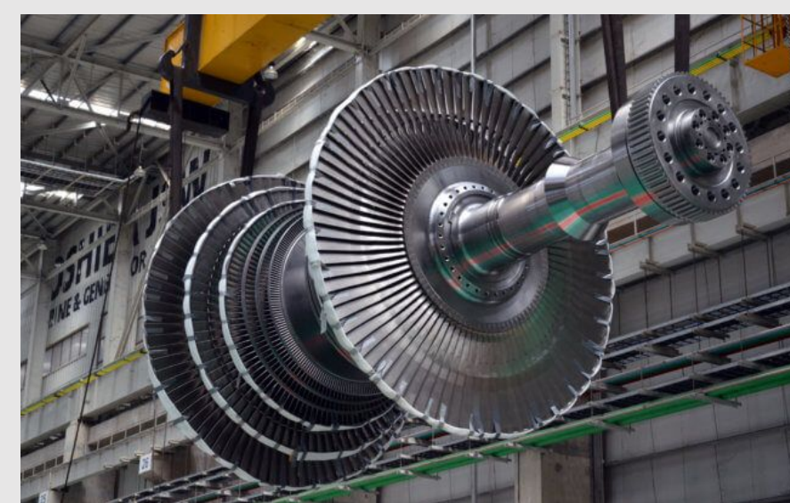
High temperature rotor for power plant [4]
