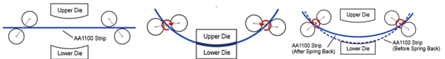
Fig 6. Diagram showing simple compression experimental procedure. Aluminum strip inserted between rollers (left), strip is bent as the rollers rotate and the upper die is lowered to apply compressive force (middle), and upper die is raised, allowing the strip to spring back.
