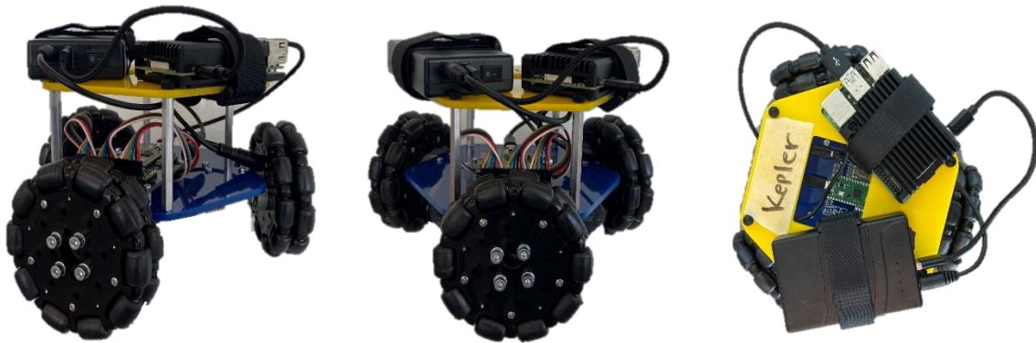
Figure 3: Fully manufactured omni-directional robot side view (left), front view (center) and top view (right).
