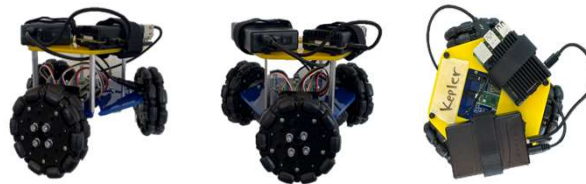
Figure 3: Fully manufactured omni-directional robot side view (left), front view (center) and top view (right).
