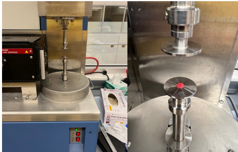
Figure 1. DMA testing setup and machine used to characterize the mechanical properties of clot analog samples.
