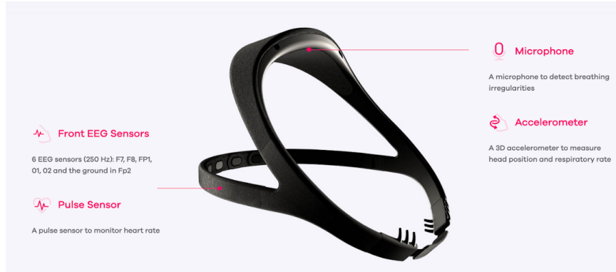
Figure 2: Dreem 2 Headband labeled with callouts showing its various sensing capabilities. Electroencephalogram (EEG) sensors are the electrodes used in PSG testing as well.
