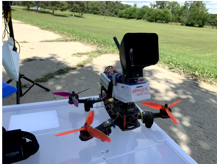
Figure 1. Mapleseed's particle collection drone, with a funnel attached to collect particles.
