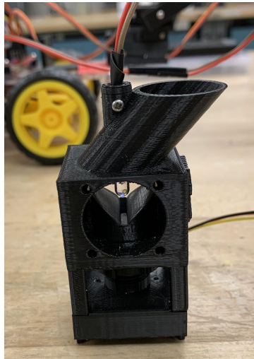
Figure 4. The microscope assembly being used for the rover and drone. The assembly includes a housing at the top with an inlet and ejection holes, a concentrator to guide the particles into the proper place, the microscope itself, and a base plate that interfaces with the rover.
