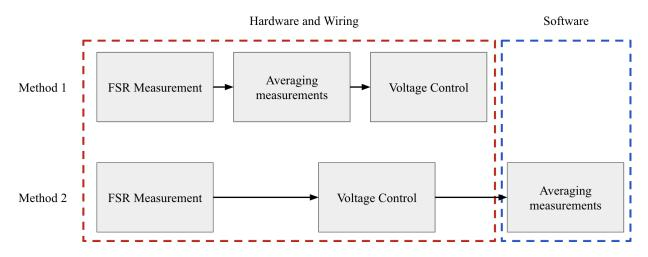
Figure 9: Differences between the two wiring systems. Blocks represent data and conversions.
