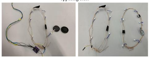
Figure 6: The electrical wiring system, without the shoes. The oblong shapes are the two copper parallels. Soldered around each edge are inserts for each sensor.
