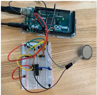
Figure 10: Current wiring system for an individual force sensor
