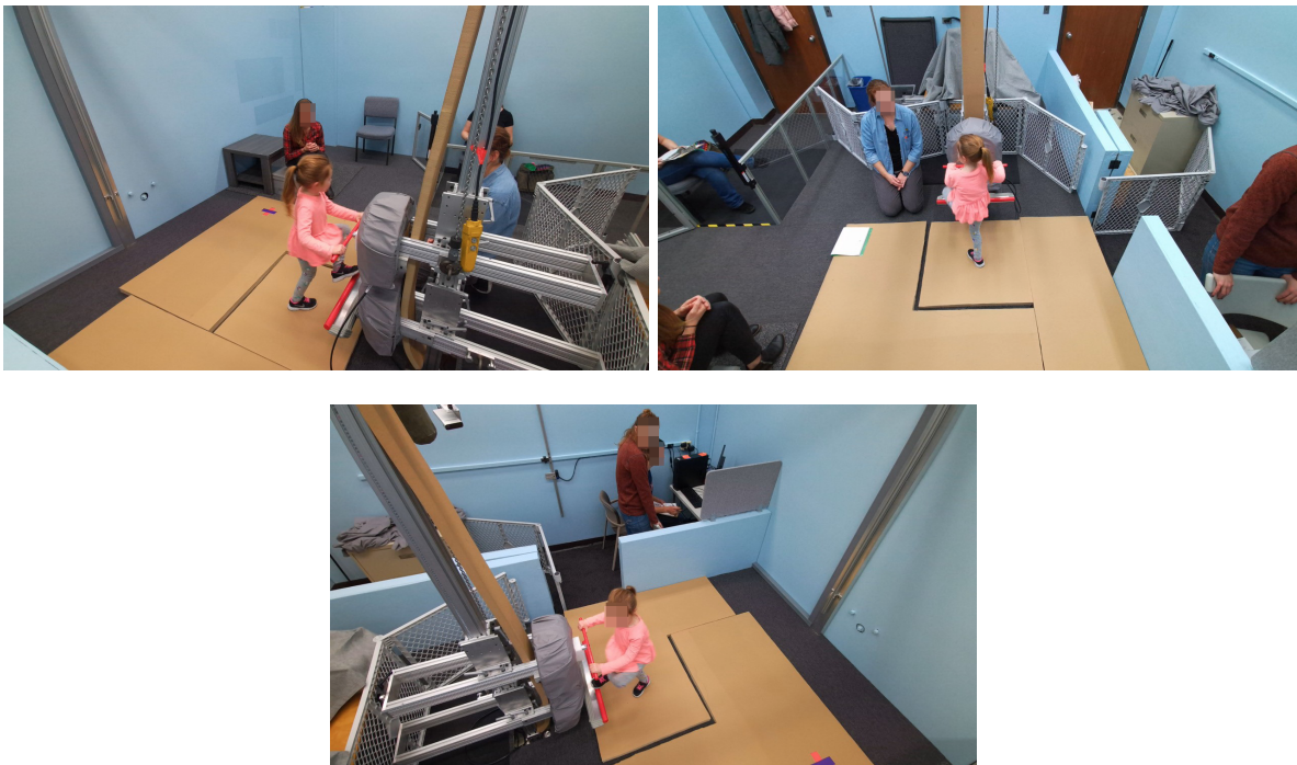
Figure 14. Examples of the RGB camera fields of view from the three Azure Kinects during data collection.
