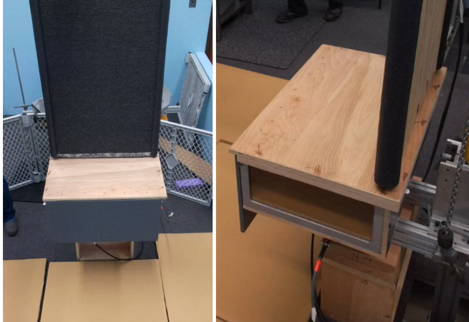
Figure 8. Photos of the table condition from two perspectives, showing the flat wood tabletop added to the box frame.
