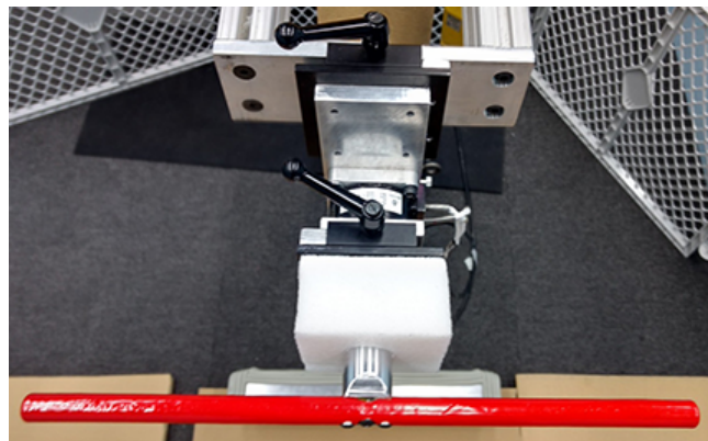
Figure 10. The handles were mounted on the 6-axis load cells via a quick release locking system. The photo shows the handle with the load cell behind it.
