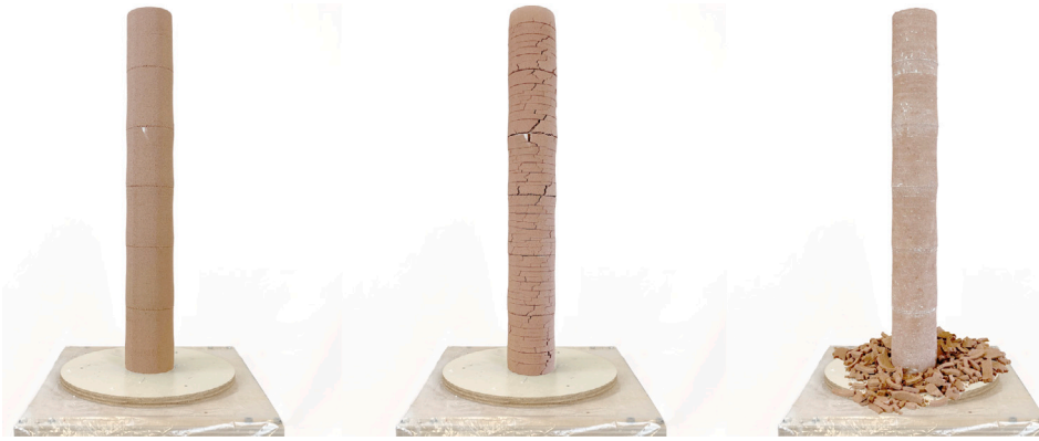
Fig. 6. From left to right: clay formwork, self-demolding dried clay, and resultant cast.
