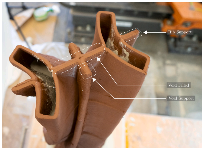
Fig. 14. Added supports facilitating the clay printing and concrete casting of the complex Cocoon element.
