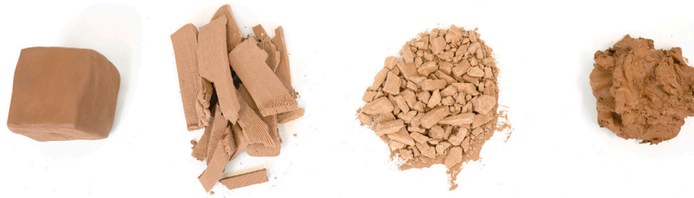
Fig. 7. From left to right: printing clay, demolded formwork, ground and separated formwork, and recycled printing clay.
