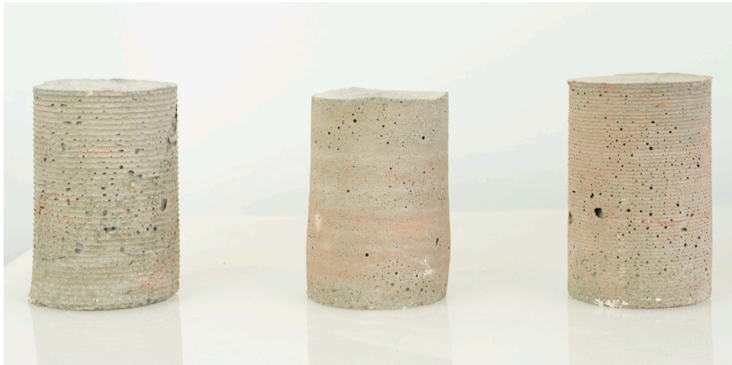
Fig. 8. From left to right: prints with 3 mm, 1 mm, and 2 mm bead heights.
