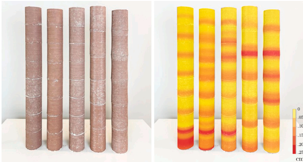
Fig. 12. Deformation control test results (left figure) and the circumferential change (right figure): (from left to right cylinder) 100 mm pour height, 20 g acc; 100 mm pour height, 20 g acc; 100 mm pour height, 30 g acc; 135 mm pour height, 30 g acc; and 135 mm pour height, 20 g acc.
