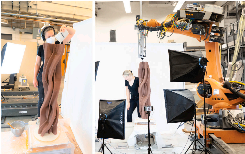
Fig. 3. Co-working environment between humans and robots, combining robotic clay printing and manual concrete casting processes.
