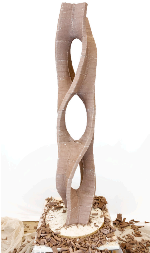
Fig. 2. Final resultant cast after demolding (height = 1.3 m).
