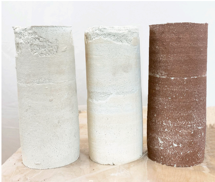
Fig. 9. From left to right: RO-95 Cone 6 Porcelain, RO-01 You Betcha Mix High Fire White Clay, and RO-82M Terracotta with Fine Grog [49].
