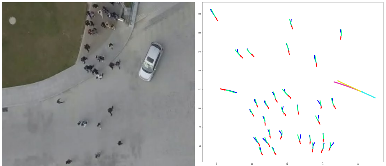
Figure 3.9 The output trajectories of the model on the DUT scenario. Left: Visual of the scene; Right: Trajectory model and prediction – Pedestrians: Red (observed trajectory), blue (ground truth), green (predicted trajectory). Vehicles: Turquoise (observed trajectory), yellow (ground truth), and pink (predicted trajectory).
