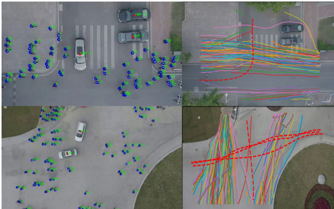
Figure 3.6 VCI-DUT Dataset with trajectories of vehicles (red dashed line) and pedestrians (colorful solid lines). Upper: Intersection. Lower: Roundabout [53].
