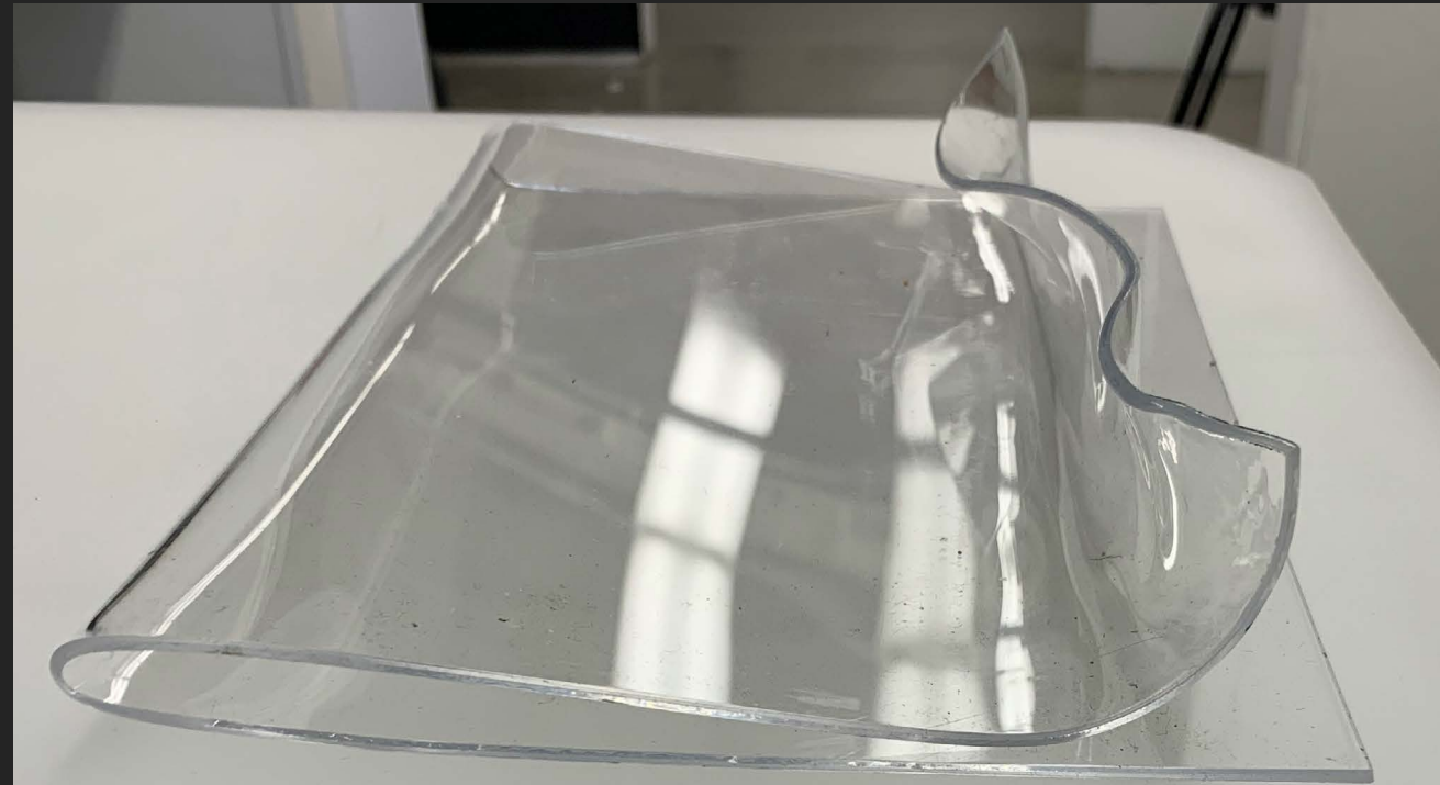
This was one of my first test on the possibility of using a heat gun to bend acrylic sheets, this test informed what sort of heat modifications I could do to my calendars.
