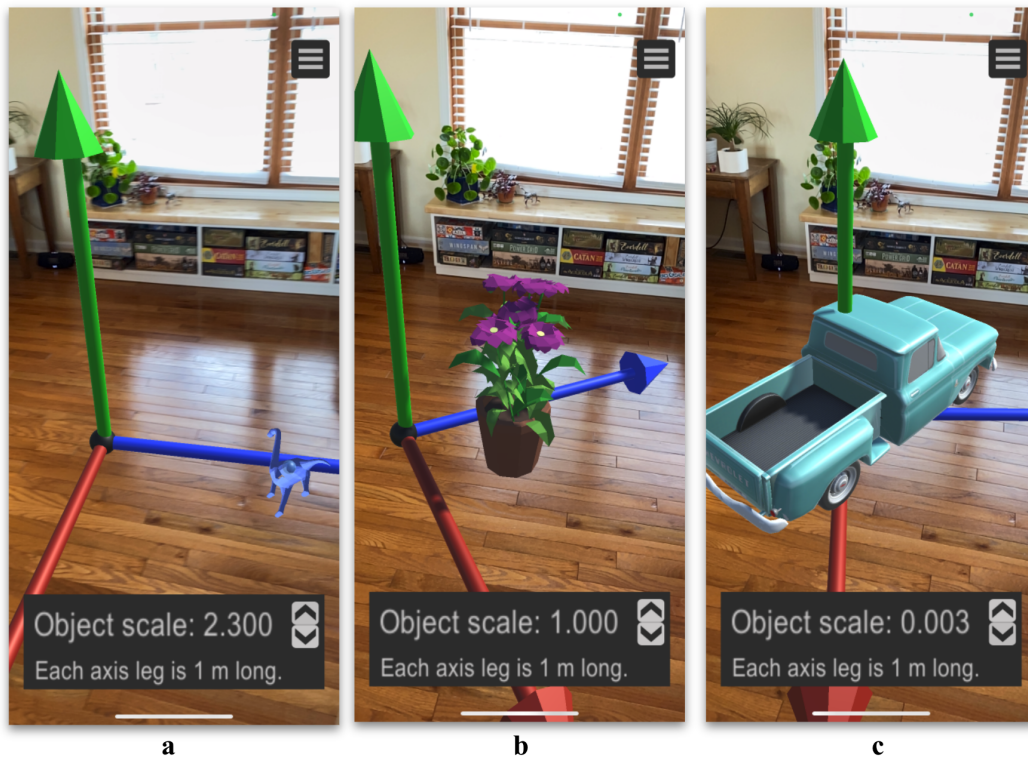
Figure 2: Sketchfab model examples: a) extremely small model (note increased scale) b) approximately life-size model c) extremely large model (note decreased scale)
