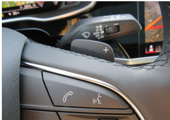
Figure 9. Example of shift paddle on steering wheel
