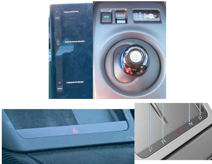
Figure 8. Example of other gear shift (slider Tesla, joystick Nissan Leaf, center console strip Tesla).
