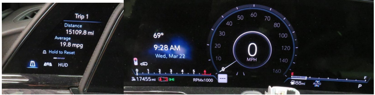
Figure 50. Two part instrument cluster on Cadillac Escalade.
