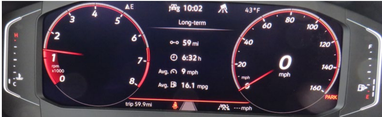
Figure 46. Primarily digital instrument clusters with simulated physical gages and separate areas for temperature and fuel gages.
