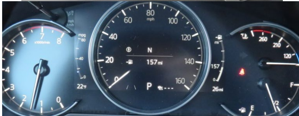
Figure 45. Instrument clusters with physical tachometer on left, physical temperature and fuel gages on right, and central digital screen including speedometer.
