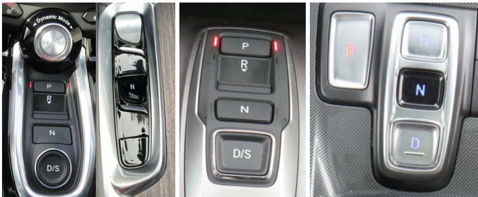
Figure 7. Examples of button gear shifts; from left to right (Acura TLX, Buick Enclave, Honda Ridgeline, Hyundai Santa Fe).
