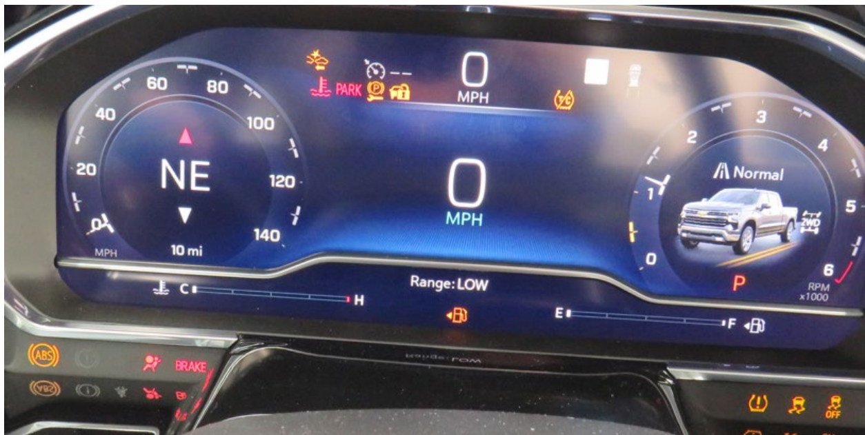
Figure 47. Primarily digital instrument clusters with simulated physical gages and separate areas for warning lights.
