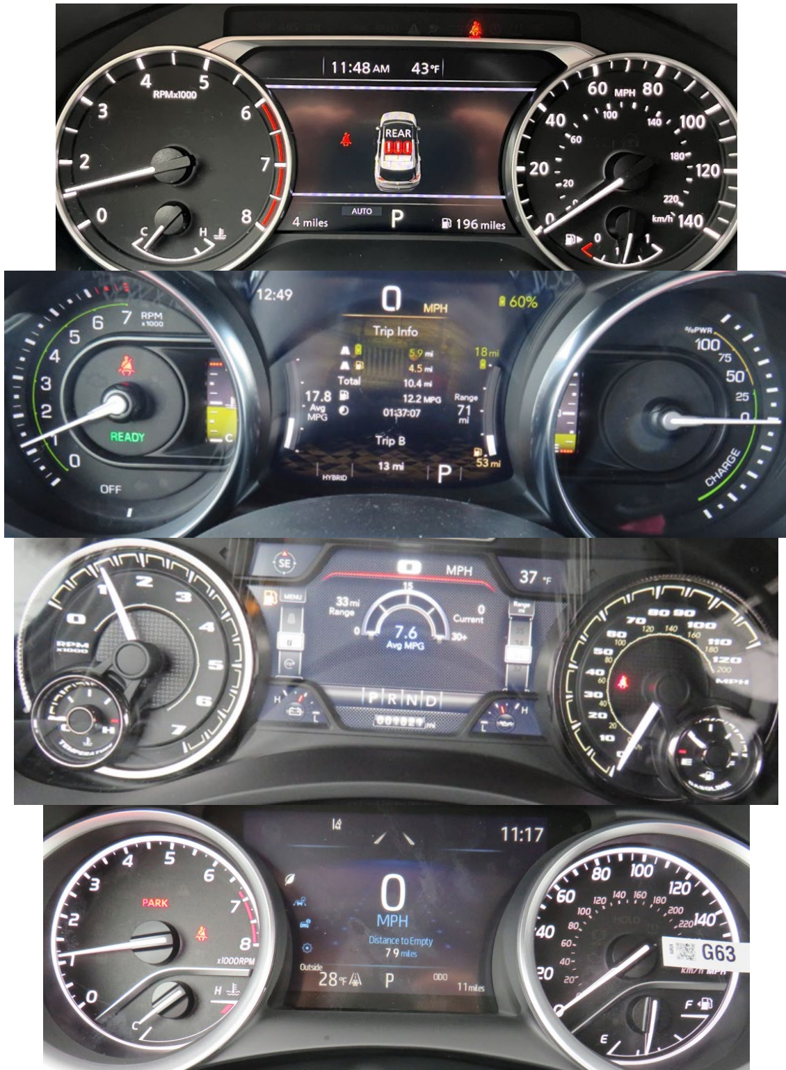
Figure 40. Physical tachometer and temperature gage on left, physical speedometer and fuel gage on right, wider or shaped central digital screen.
