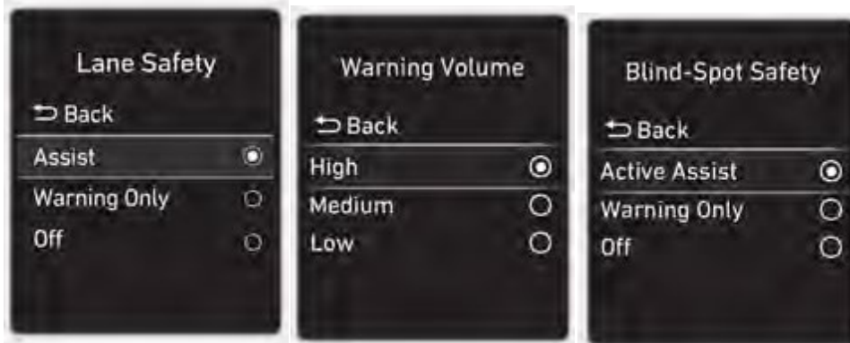
Figure 32. Examples of Warning System Settings in the Instrument Cluster (Hyundai, Kia Specifically)
