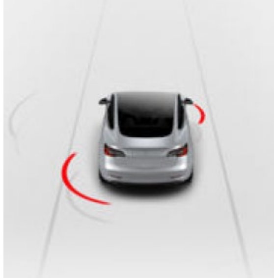
Figure 17. Tesla Y blind spot camera view; colors change with proximity.
