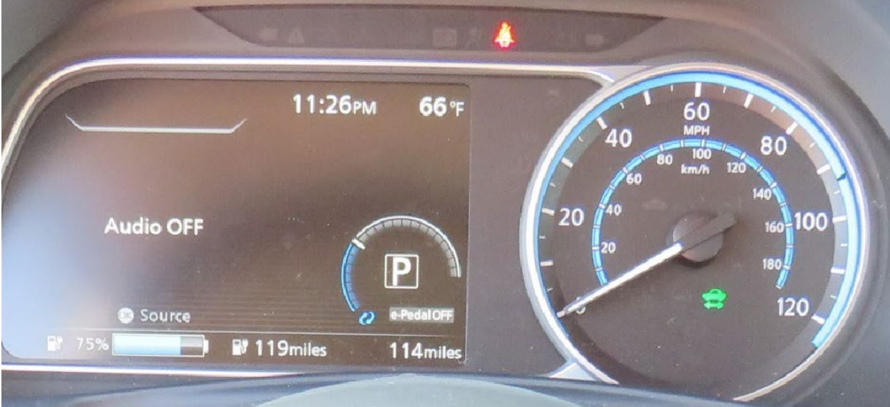
Figure 43. Instrument cluster with screen on the left and physical speedometer on right, plus upper warning screen.
