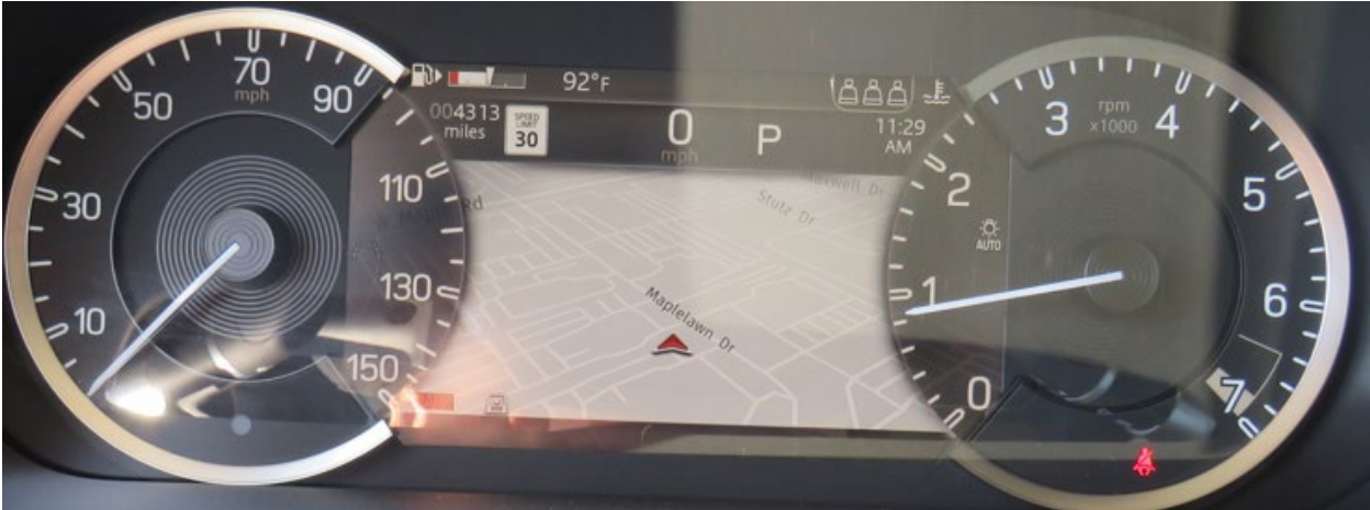
Figure 44. Instrument cluster with physical speedometer on left, physical tachometer on right, and wider contoured center screen including map feature.
