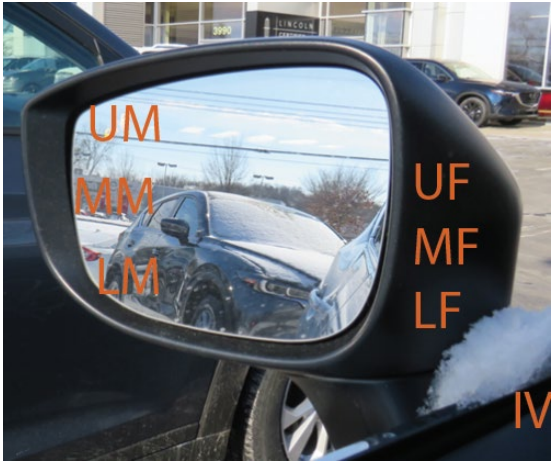
Figure 16. Examples of locations where blind spot warning telltales appear. Upper mirror (UM), middle mirror (MM), lower mirror (LM), upper frame (UF), middle frame (MF), lower frame (LF), inside vehicle (IV).
