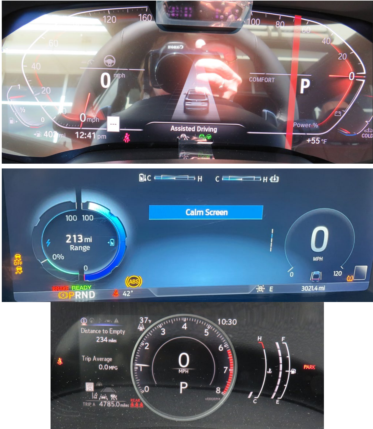
Figure 49. Digital instrument clusters with simulated nontraditional gages.
