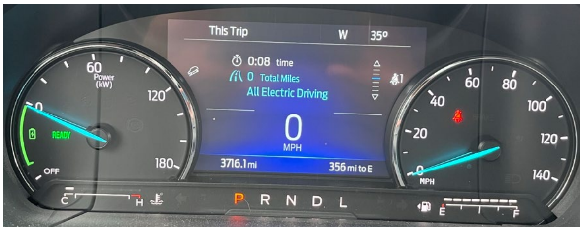
Figure 42. Instrument cluster for hybrid vehicle with physical power gage on left, physical speedometer on right, and digital screen in center.
