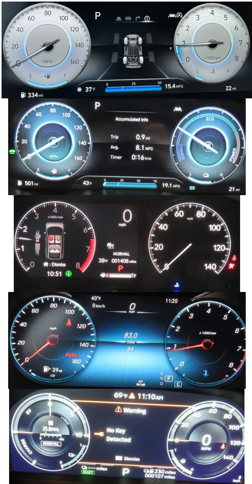
Figure 48. Digital instrument clusters with simulated traditional gages.
