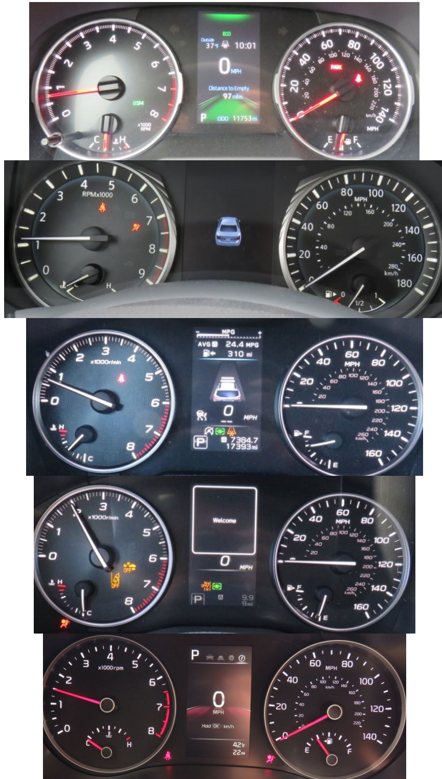
Figure 39. Physical tachometer and temperature gage on left, physical speedometer and fuel gage on right, narrow central digital screen.
