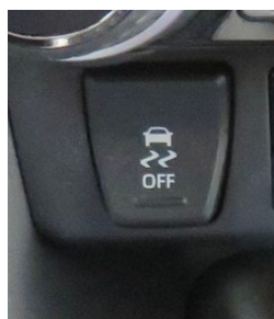
Figure 14. Example of typical ESC shutoff control.
