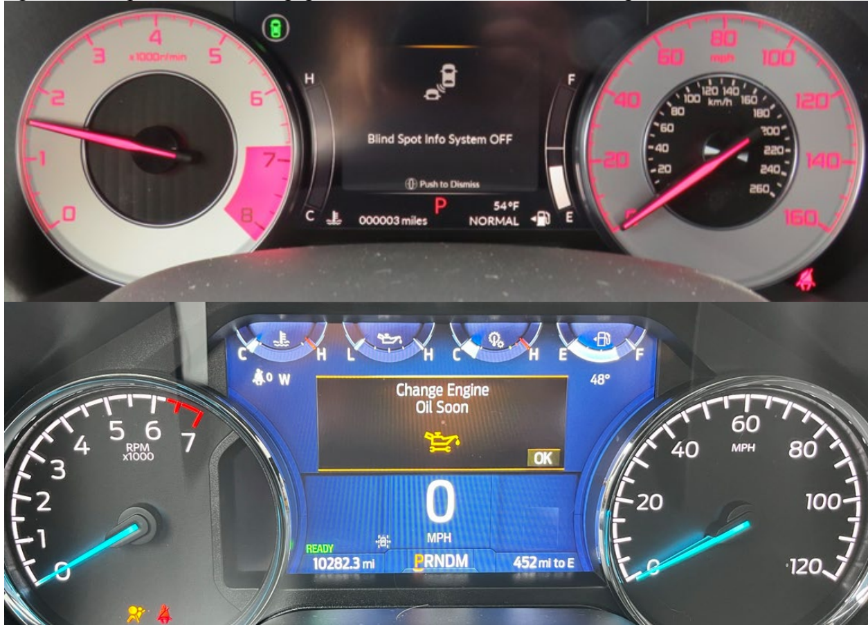
Figure 41. Instrument clusters with physical tachometer on left, physical speedometer on right, digital screen including temperature and fuel gage in center.
