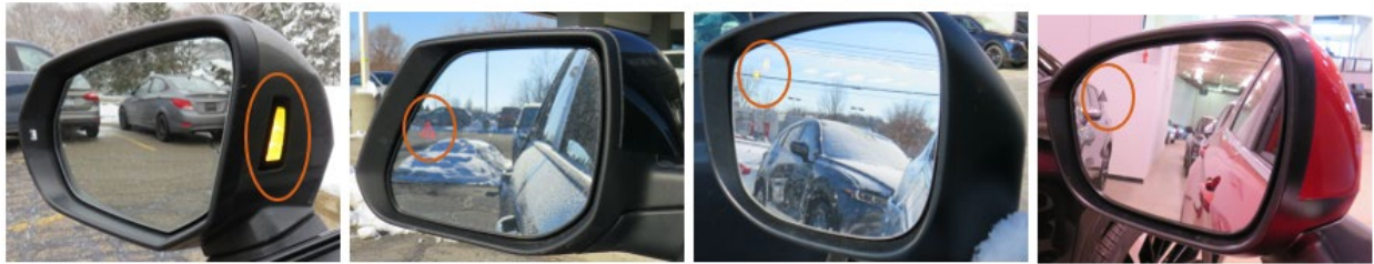
Figure 15. Examples of blind spot warning telltales: light, hazard symbol, ISO symbol, triangle.
