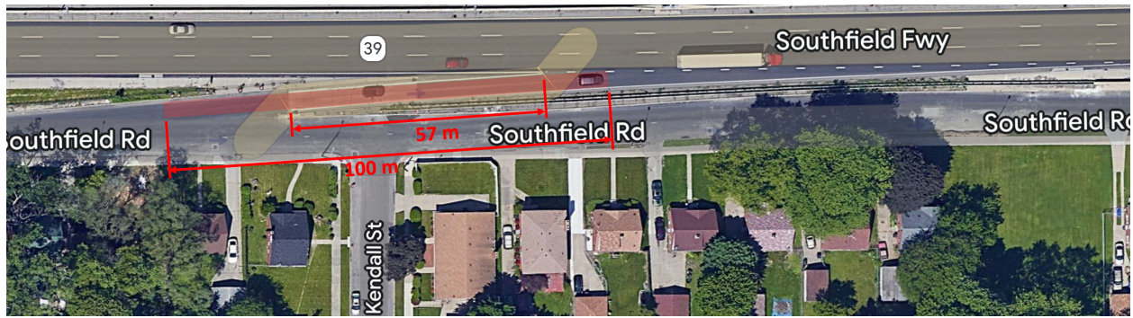
Figure 4: Real-world view of a highway merge on-ramp copied from Google Maps, March 6, 2023. Overhead view of the Southfield Freeway near Schoolcraft Road in Detroit, Michigan. The end of the red highlighting is the goal position. It is where the merge lane width becomes narrower than a standard lane width. The pictured on-ramp merge lane length is estimated at 100 meters. The vehicle at the end of the ramp has nearly reached the goal. A 57 m length is marked between the end of the painted lines within the merge lane and correlates to the same measurement shown in Figure 5.
