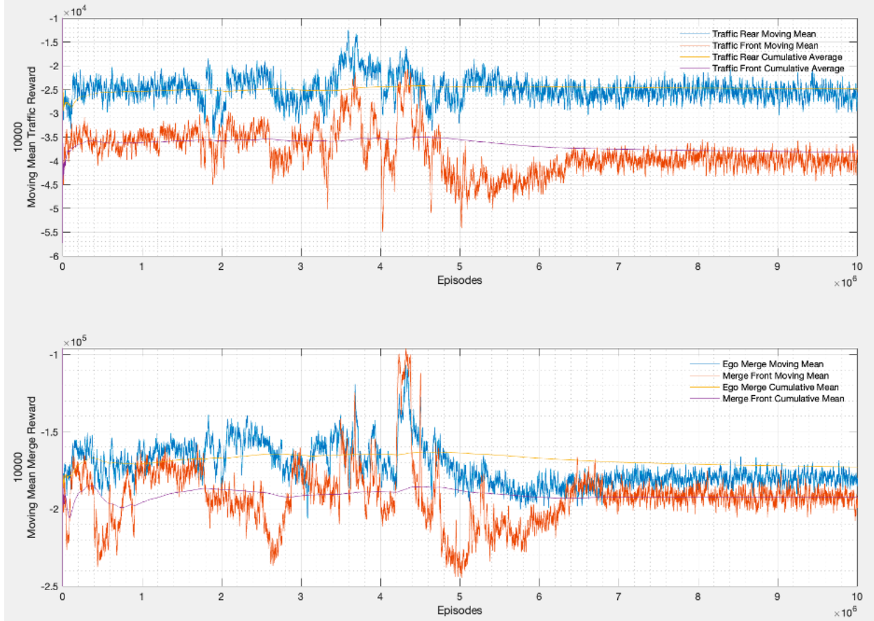
Figure 55: Training graph of moving mean and cumulative average for rewards. Data in the lower graph is for both front and rear merge vehicles. The upper graph shows the closest front and rear traffic vehicles to the rear merge vehicle. Near seven million episodes, the acceleration action for both the merge and traffic vehicles settle to continuously choose an action limit value of -5 \text{ m/s} acceleration, regardless of the state value.
