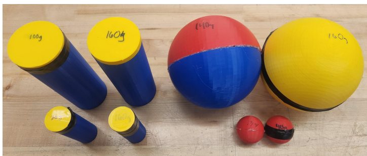
Figure 11.5 3D-printed testing specimens. The cylindrical objects represent the contaminants while the spherical ones represent the compost wastes. The size and weight of the specimen are chosen according to the engineering verification thereof specified.
