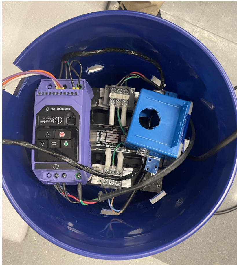
Figure 21. Full electrical setup contained within our modified Lowe's paint bucket. The transformer is located at the base of the bucket. The motor controller (purple) and additional wire housing (blue) were placed on top of the transformer for easy access. No wires are strained in this configuration. The electrical box is covered with a lid during normal operation to eliminate the risk of touching any live components.
