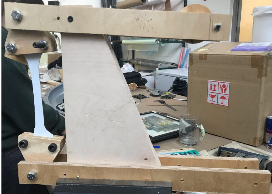
Figure 28. An image of our built miniature tensile tester. Includes an ABS sample inside the grips.
