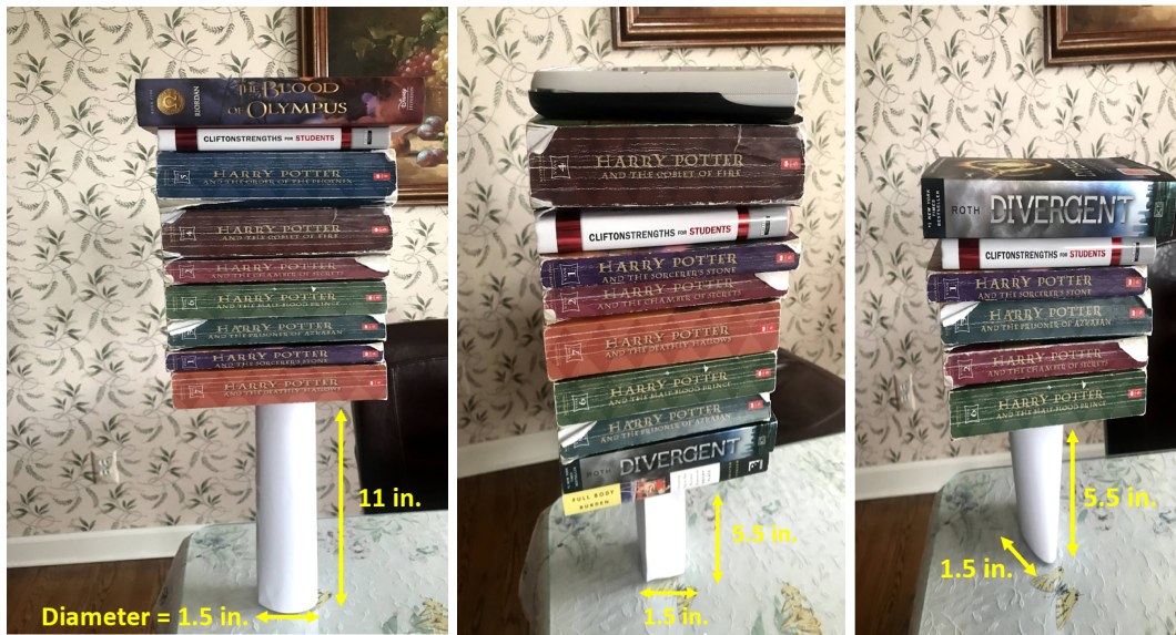
Figure 18. The three images shown are the first prototypes of the paper columns activity. The images from left to right show: (1) a long circular column, (2) short square column, and (3) a long triangular column.
