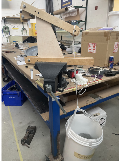
Figure 36. An image of our tensile tester with weight in a bucket hanging off the lever with a broken ABS sample.
