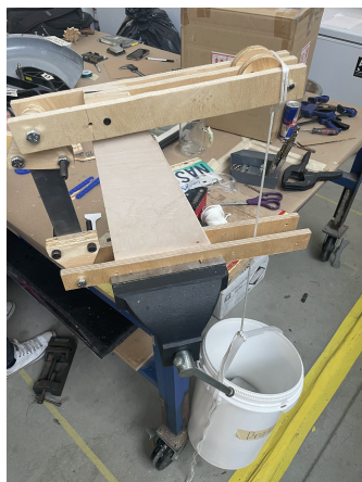
Figure 37. An image of the setup of the tensile tester.
